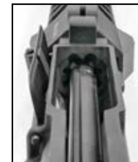
Insert scraper into star chamber and twist to scrape
